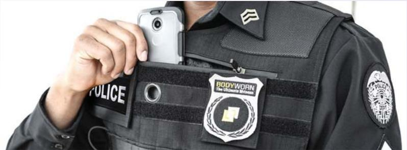
turn them on and off by tapping on their chest. Officers will also have a bluetooth enabled wristband that they can touch to activate the camera. A router, called "The Rocket" will transfer the video recording in the trunk and when the patrol car returns to the station, the data is uploaded into the Cloud, where the footage can be reviewed instantly.
